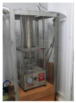
Figure 3. Potter-Precision Laboratory Spray Tower
