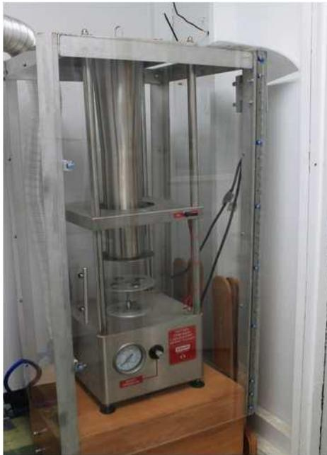
Figure 3. Potter-Precision Laboratory Spray Tower
